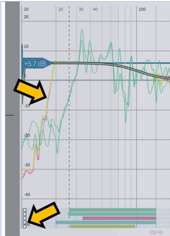
Figure 1: Bass response with infra bass bypass option disabled.
